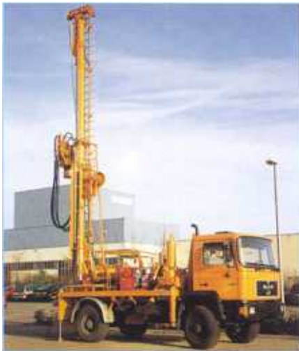
rig in drilling position
