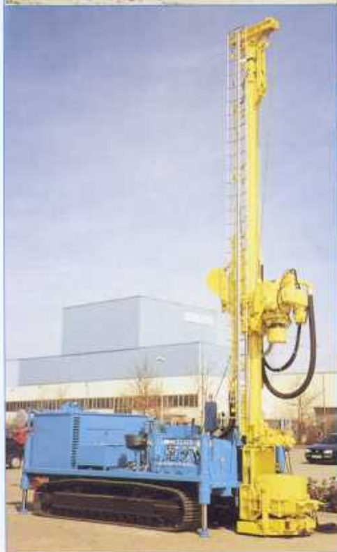
DSB 2/10 on crawler B2 incl. casing rotary table. Rig in transport and drilling position.
