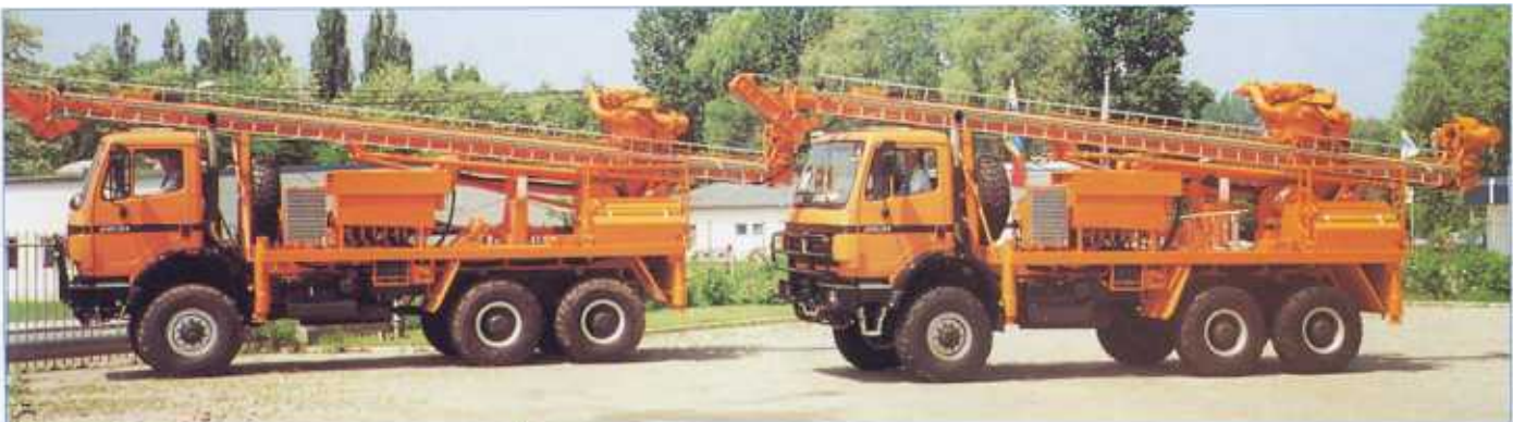
DSB 2/10 on Mercedes 3-axle-truck all-wheel-drive -2631 AK/6 x 6- as water well drilling rig.
