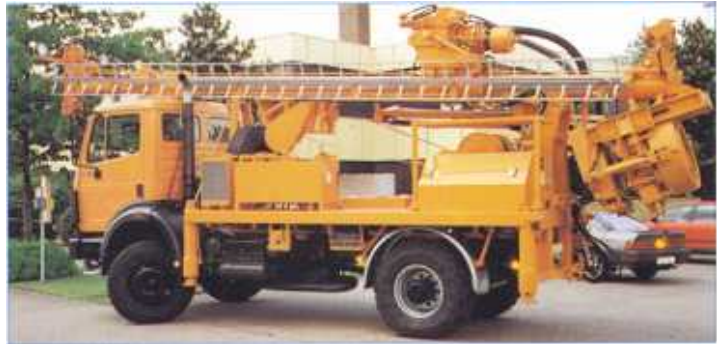
DSB 2/7 in driving and transport position on Mercedes truck -1824 AK- including hydr. casing rotary table folded down for transport.
