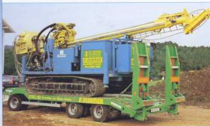
DSB 2/10 on crawler B2 incl. casing rotary table. Rig in transport and drilling position.
